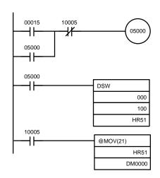
When IR 00015 turns ON, the IR 05000 will hold itself ON until the One Round Flag (IR 10005) turns ON upon completion of one round of reading by DSW(—).
